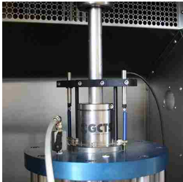
Figure 3.19 External LVDT Setup Clamped to Loading Piston
