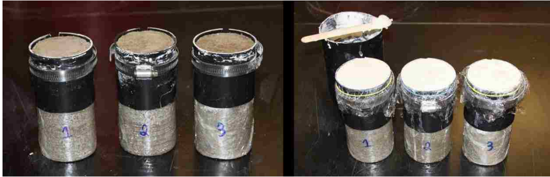
Figure 3.10 Example of Gypsum Cement Capping Method
