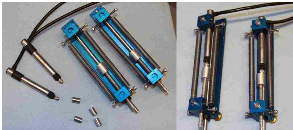
Figure 3.16 LVDT Setup for Glued Button Deformation Measurement
