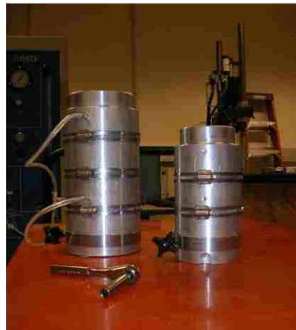
Figure 3.8 Split Molds Used for Compaction
